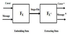
Fig. 1: Structure of Steganography System
